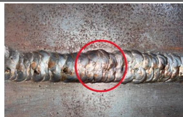
Figure 10. Welding Defects (Overlap) on Welding Workpieces (MIG) 2
