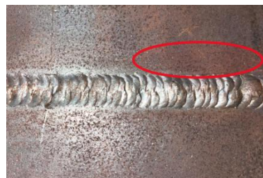
Figure 12. Welding Defects (Spatters) on welding workpieces (MIG) 3
