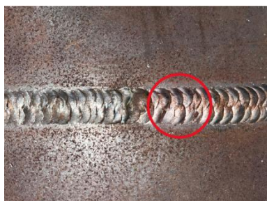
Figure 13. Welding Defects (Overlap) in MIG Welding Workpiece 3
