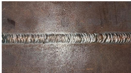
Figure 4. Welding Workpiece (MIG)3 (S3)
