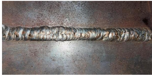
Figure 3. Welding Workpiece (MIG)2 (S2)
