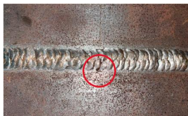
Figure 11. Welding Defects (Undercut) on Welding Workpieces (MIG) 3
