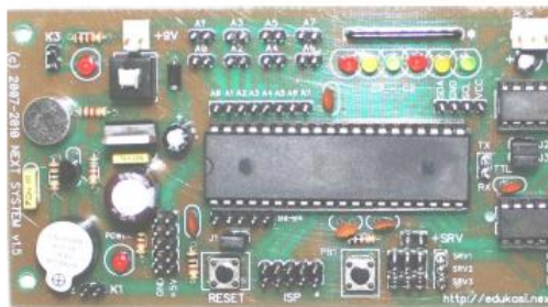
Gambar 17. Rangkaian Board Controller Robot
