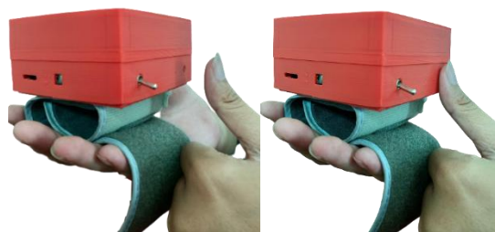
Figure 6. Example of incorrect temperature measurement due to fingers too far and too close to the temperature sensor (MLX90615)
