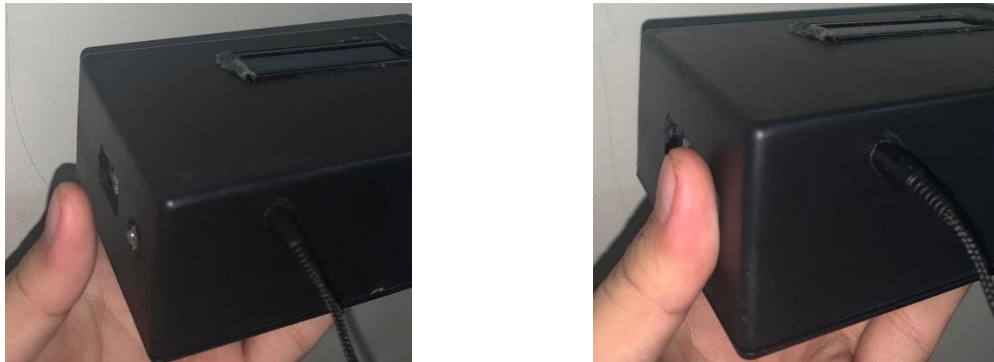
Figure 6. An illustration of inaccurate temperature measurement caused by fingers being positioned both too distant and too close to the temperature sensor (MLX90614)
